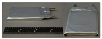
Figure 2: Photo showing the 1.5 Ah High-Power, Low-Temperature Li-Metal Battery Cell
