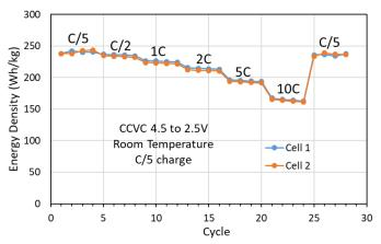
Figure 5: Energy density as a function of discharge rate
