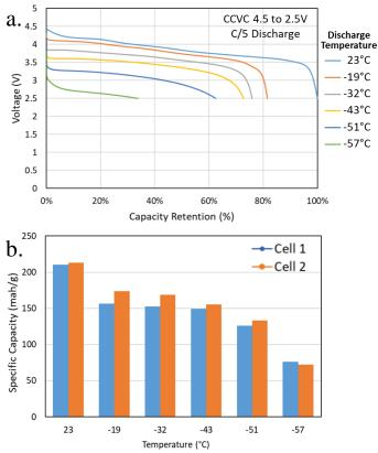
**Figure 3:** a) State of discharge profiles (voltage vs capacity retention) for cells discharged at different temperature. b) Specific capacity of the cathode active materials at different discharge temperatures.
