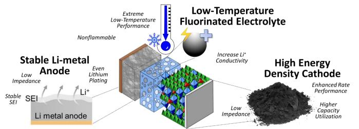
Figure 1: Illustration of the High-Power, Low Temperature Li-Metal Battery Cell for military applications
