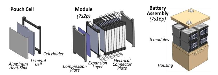
Figure 6: CAD model integrating High-Power Li-metal cell into 6T battery platform
