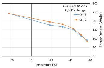
Figure 4: Energy density as a function of temperature.
